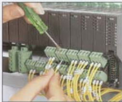
The slanted I/O terminals are easily accessible even with high-density wiring.
